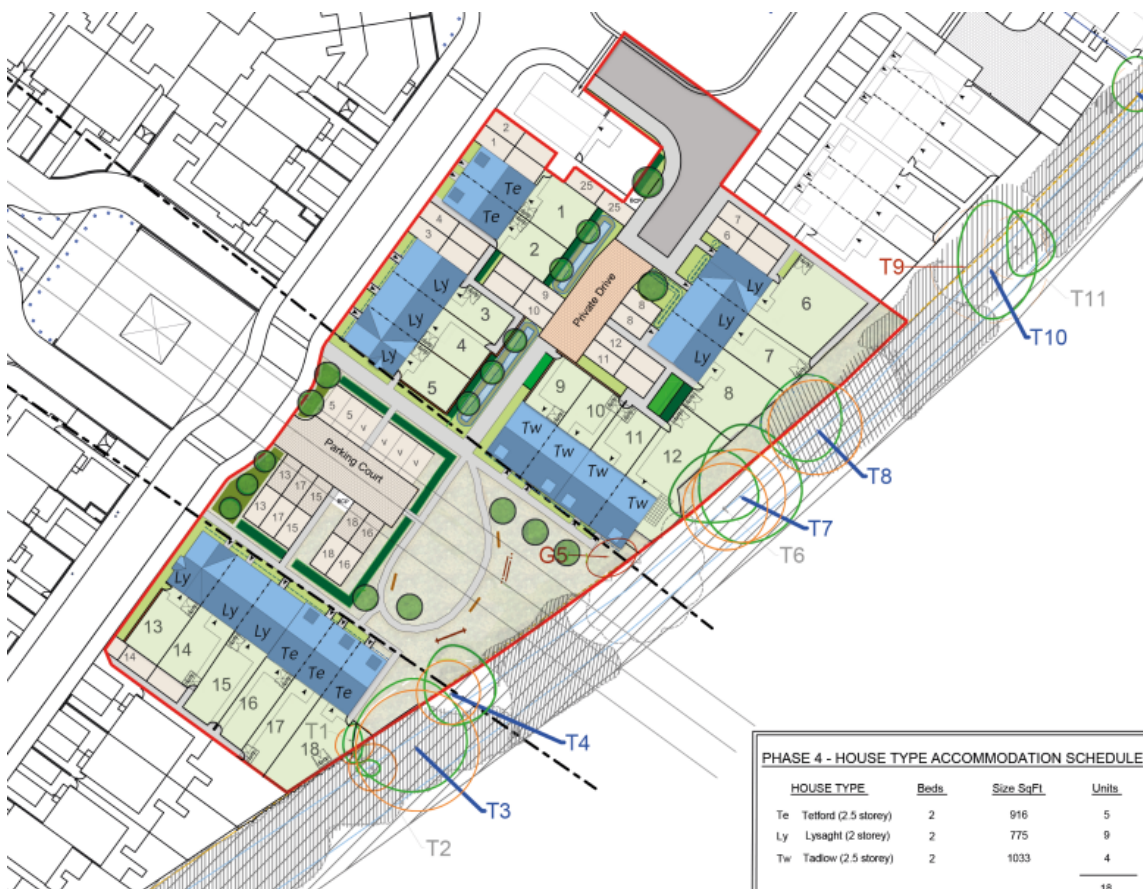
Extract from proposed site layout drawing noting 2m wide footpath around turning head north of site, increased width of footway connecting northern and southern parts of the site and individual cycle storage sheds for each unit.
